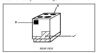
To move the appliance, open the fan oven door, and lift the appliance by holding inside the top of the compartment.
